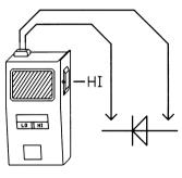
a díode has a break or a short. The same applies to light-emitting diodes (LED's). Zener or Z-diodes also deliver a tone in the non-pass direction up to about 5V zener voltage. But this tone is significantly deeper than in the forward direction.
